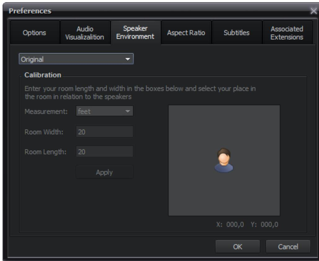
The number and configuration of speakers is selected from the upper drop-down box. The speakers will be displayed schematically together with the user position in the room:
